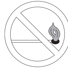
Fig. 3 – Do Not Light Burner with Match
